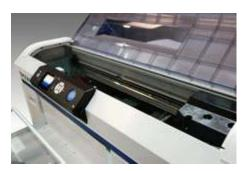
Top Access Cover: Allows for easy access for printer maintenance and for viewing garments being printed. The cover is open in this photo.
