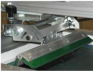
• **Dual Action Squeegee:** Uses a dual-action (flip-flop), industry standard, aluminum squeegee holder to ensure long-lasting screens and maximum versatility. Allows you to print and flood with the squeegee blade (sharp, round or semi-round) as the print job specifies.
