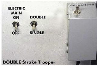
• **Double Print:** This option gives you the capability of simulating manual printing where you want a double-print stroke on the first print head. Flip a switch and Head #1 will stroke twice.
