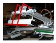
• The Equalizer Print Head (patent pending): Gives you the capability of adding an extra print head to the Mini-Trooper without sacrificing your load/unload station area. Features a clamshell design. Pivots the print head up and down automatically in sync with the print cycle of the press. Saves space - when not in use, print head remains in the up position.
